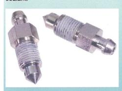
Applying a sealant to a brake bleeding nipple or union thread will seal the thread from moisture and deter future corrosion. It will also stop the leakage of air or brake fluid past the thread of the open brake bleeding nipple while bleeding. Note, when applying thread sealant, allow the first two threads above the bleed bleeding nipple 'point' to be sealant free and do not over tighten.
